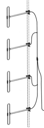
Quarterwave Spacing Horizontal
