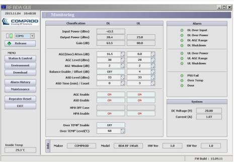
Visual Alarms and Remote Failure Monitoring with Graphical User Interface
