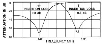
504-90 Typical Response Curve at 5 MHz Spacing
