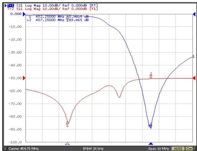
506-90 Typical Response Curves at 5 MHz Spacing
