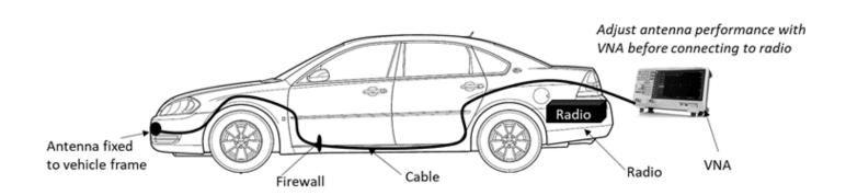
2.2 After cable installation, use a VNA (Vector Network Analyzer) to ensure that the antenna is performing in customers frequency band (central frequency, operating bandwidth & VSWR). No tuning is required.
