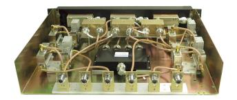
\*These are generic pictures of the control station combiner. The size of components used for the VHF version, will depend on required frequencies.
