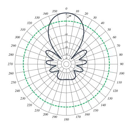
(2)987-70 Horizontal radiation pattern, Vertical polarisation,
