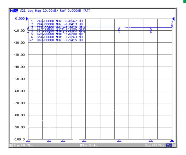
Typical test results of ANT-RX Insertion Loss
