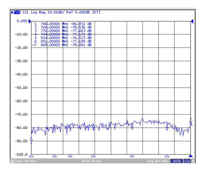
Typical test results of Radio1-Radio2 Isolation
