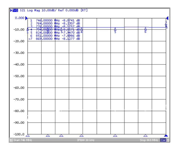
Typical test results of TX-ANT Insertion Loss
