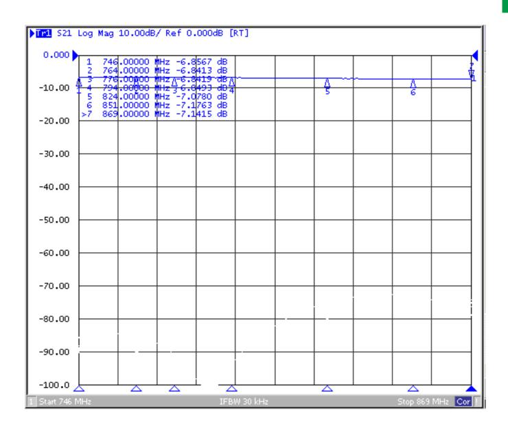
Typical test results of ANT-RX Insertion Loss
