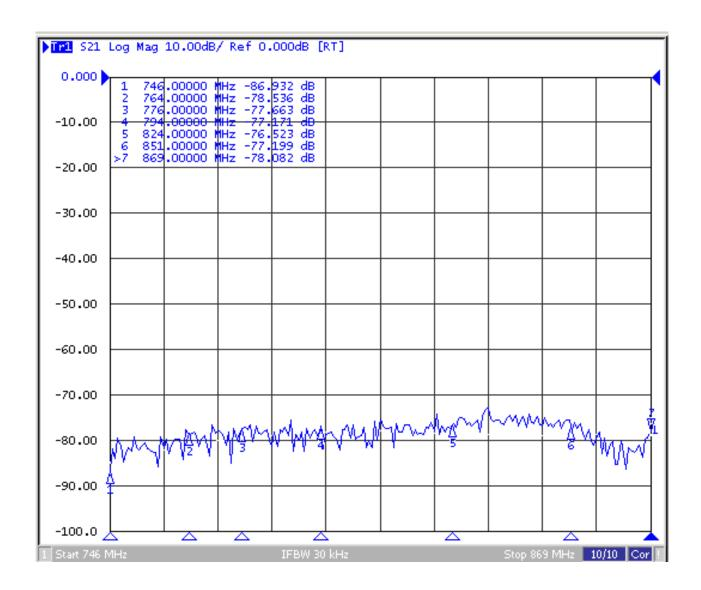
Typical test results of Radio1-Radio2 Isolation
