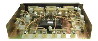
\*These are generic pictures of the control station combiner. The size of components used for the UHF version, will depend on required frequencies.
