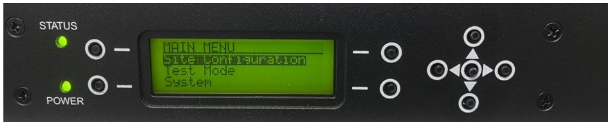
Fig. 6 BTS C&DU configuration via Front Panel
